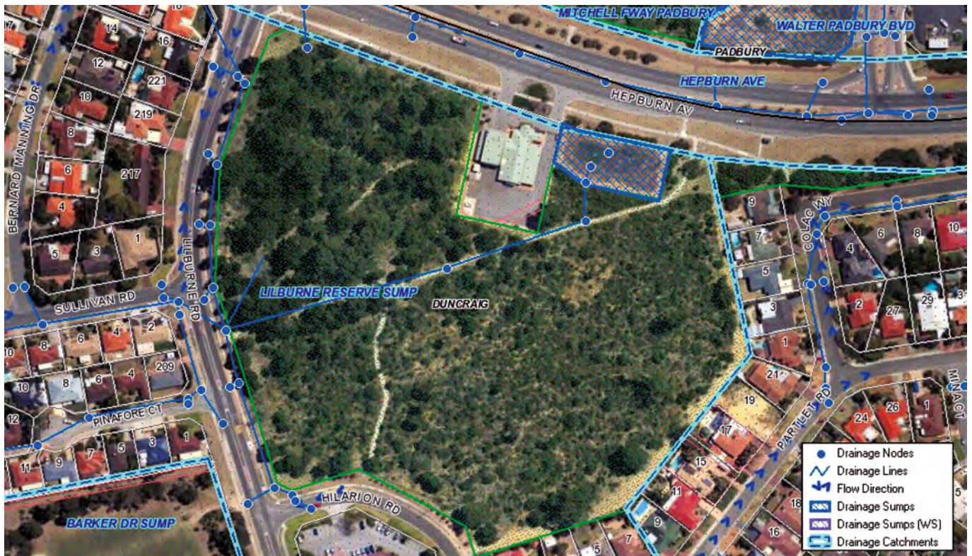
Figure 7: Lilburne Park Drainage Lines and Sump
