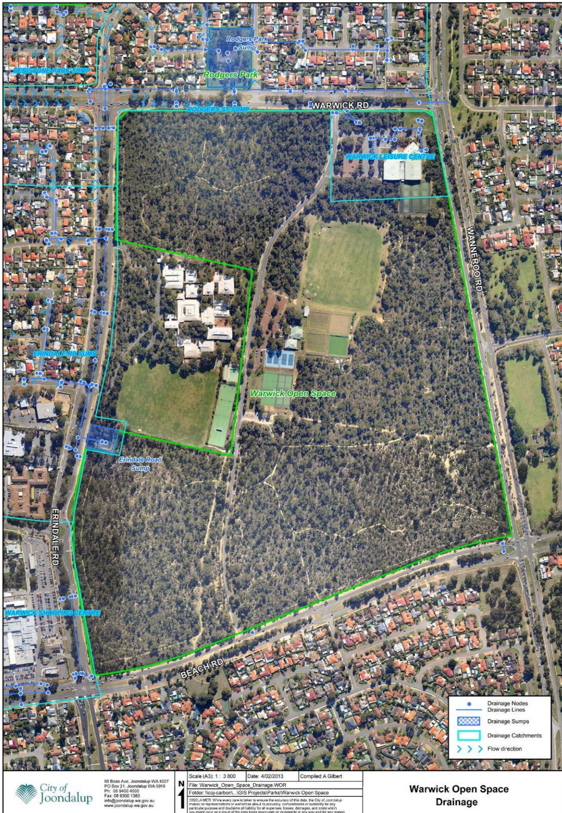
Figure 9: Warwick Open Space Drainage Lines and Sump
