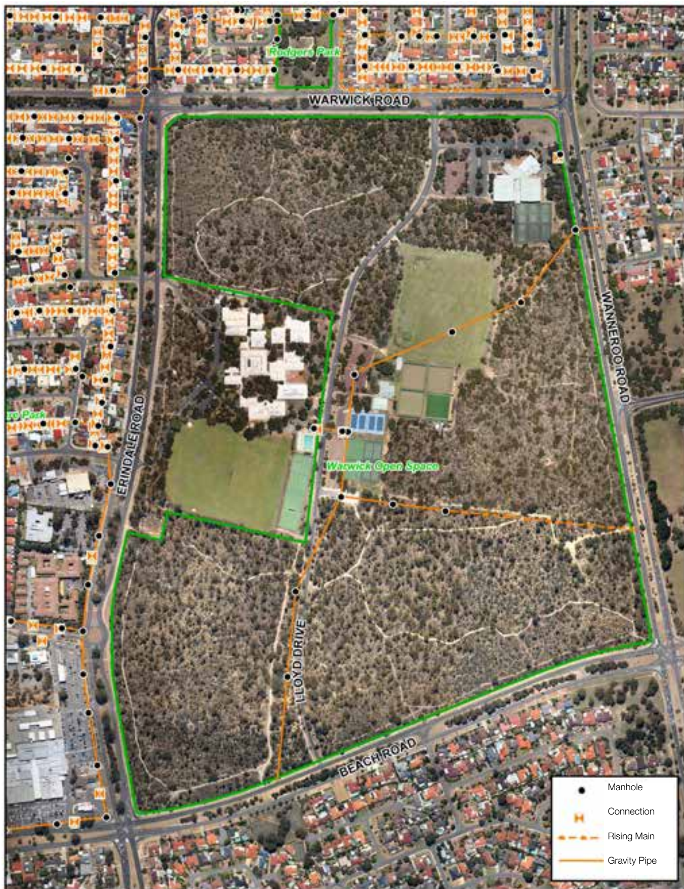
Figure 26: Warwick Open Space Sewerage Utilities
