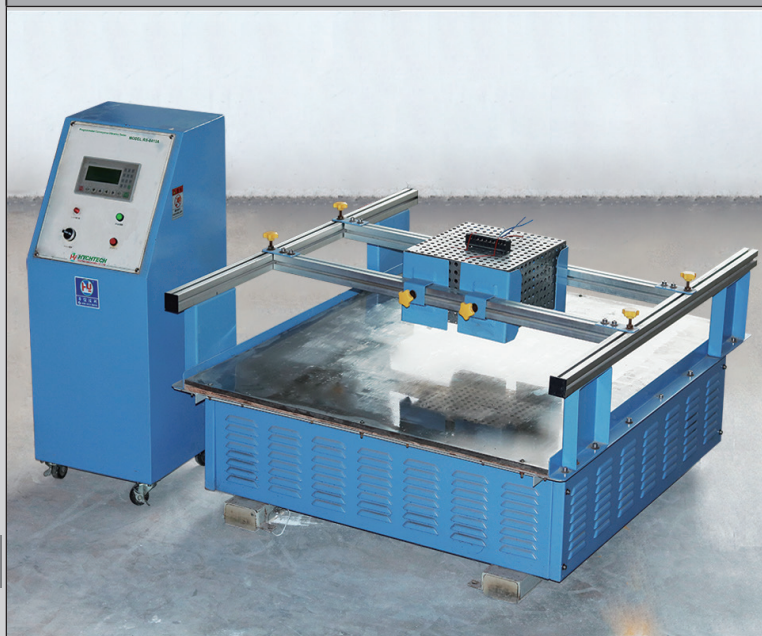
Vibration test equipment
