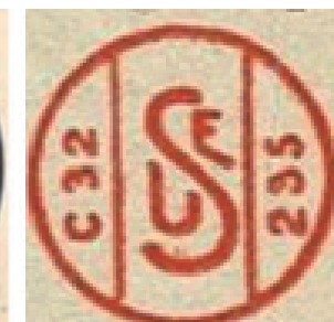
1957 Marking USE printed with the standard number (C32) and the manufacturer identification number (295)
