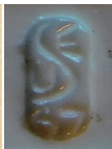
1932 ca USE marking on Maure porcelain terminal blocks
