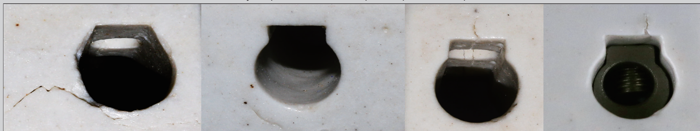
Examples of cracks on C111 porcelain
