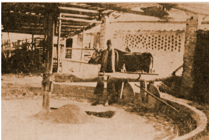
Grinding of kaolin by grinders powered by an ox (1939, Vietnam, Economic Bulletin of Indo-China)
