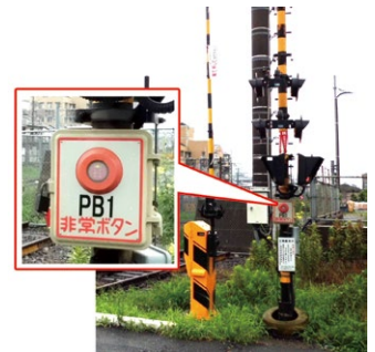
Level crossing alarm system
