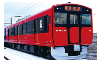
EV-E801 series Accumulator railcar train for use on alternating current (AC) section
