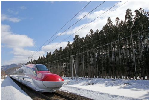
Sashimaki No.1 railway forest on the Tazawako Line (forest to protect against blizzards)
