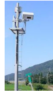
Three-dimensional laser radar obstacle detection method (large obstacle detector)
