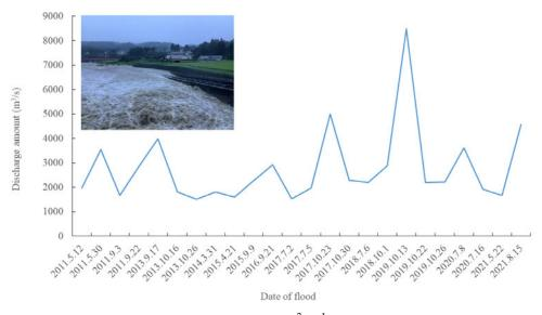
**Figure 2.** Records of discharges of over 1500 m<sup>3</sup> s<sup>-1</sup> from 2011 to 2021. The photo shows the situation of approximately 4500 m<sup>3</sup> s<sup>-1</sup> discharge at the time. The curved section of the fishway was clearly submerged.
