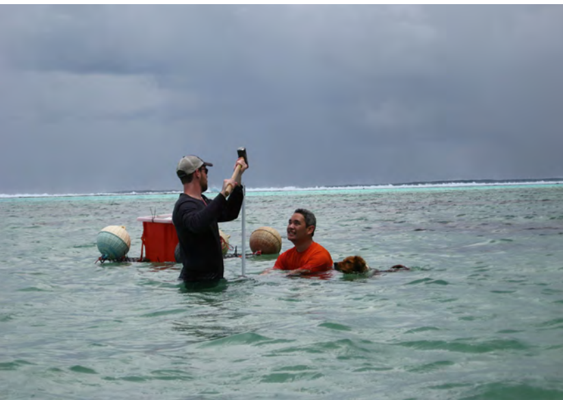
Clockwise from top left: Kevin Befus (left) and Bayani Cardenas install piezometers and thermistors in Muri Lagoon to look for signs of groundwater flow; reds and oranges in electrical resistivity data from Muri Lagoon indicate possible presence of fresh groundwater and nutrients, likely a result of sewage from the island's human population and pig farms; the team prepares to conduct a boat-towed ER survey of Muri Lagoon from an experimental, pedal powered catamaran; Kevin Befus shows school pride.
