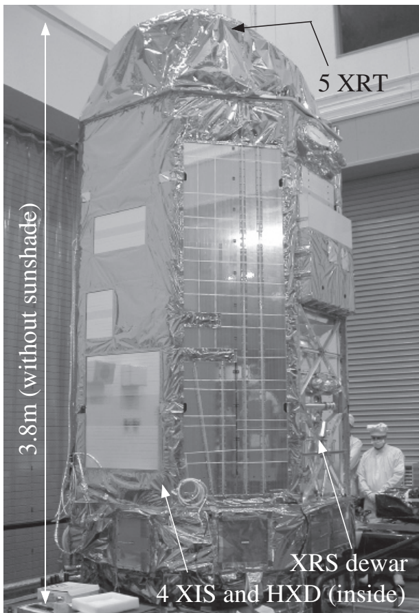
Fig. 1 A photograph of the Astro-E2 spacecraft during the thermal-vacuum test at ISAS.
