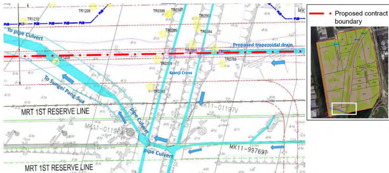
Figure 37: Proposed layout of trapezoidal drain and its connection to the unlined earth drain on the east of Kranji Cross (Source: CPG)
