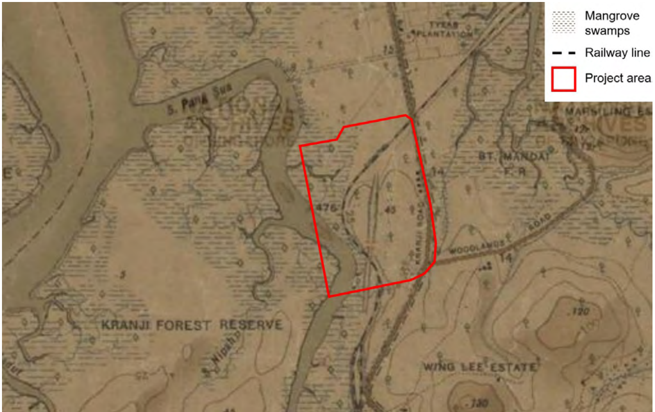
Figure 3: Topographical map of the Project area in 1924, showing that most of the Project area was dominated by mangrove swamp. The planned alignment of the railway is also shown (National Archives of Singapore, 2019).
