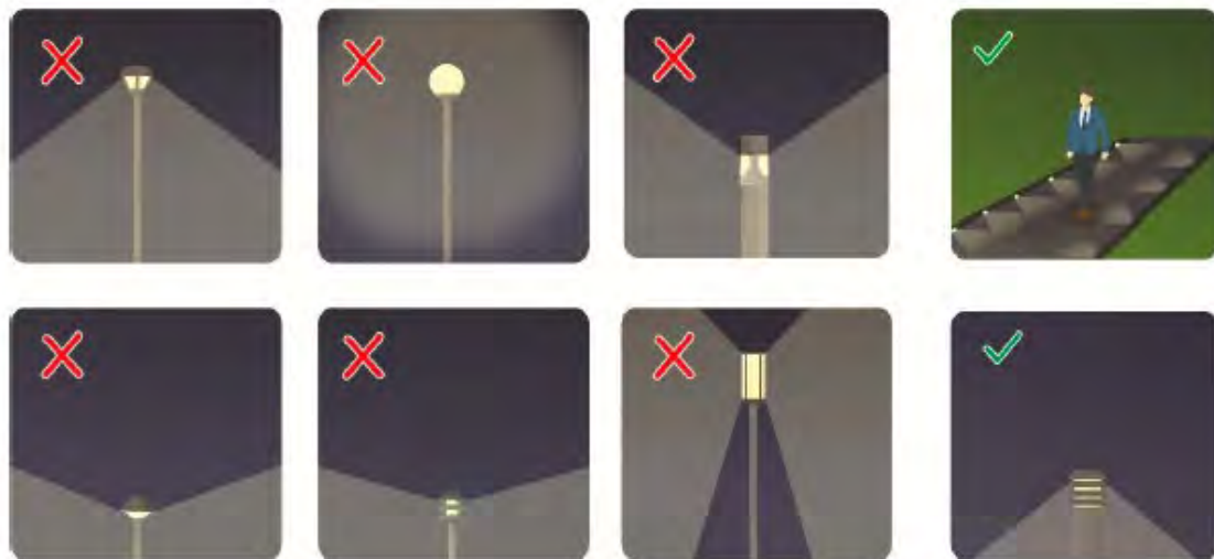
Figure 48: Walkway lighting should be mounted as low as possible and shielded. Figure adapted from Withering & Martin (2003)
