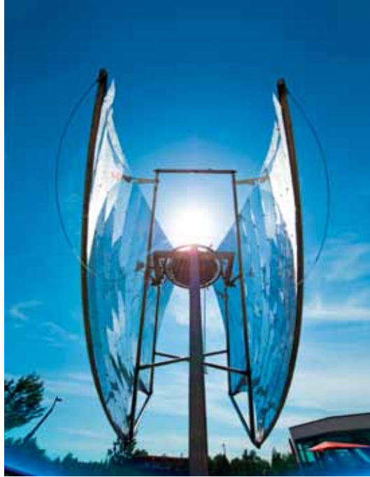
(Folded up) Papillon solar cooker of the Jülich Solar Institute
