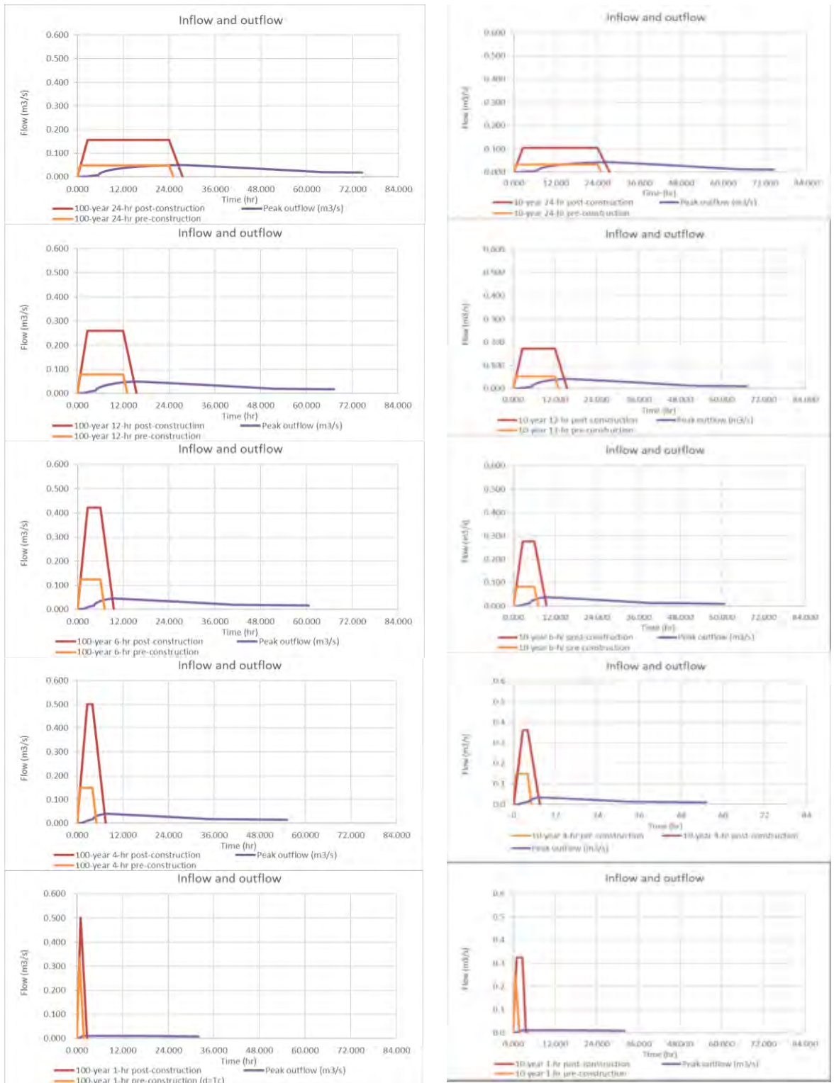
Figure 4: Pond 4 100 year and 10-year ARI discharge including climate change for pre and post development hydrographs
