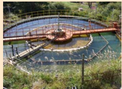
Drainage treatment facility to which the slime-filtering method is applied (reservoir tank at the Oya Mine)
