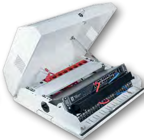
Application example 2: 19" level is angled, 3U with mounting depth up to 140 mm and 4U rear sided are usable
