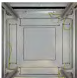
Cabinet bottom with pre-installed earthing bar, surrounding cable entries and pre-punched cutout 380 x 380 mm
