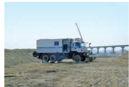
Soil strata survey using the Geo-Explorer truck
