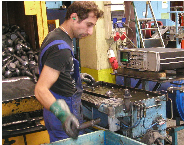
Figure Testing Setup. Existing setup with manual feeding and analogue multi-channel electronics.
