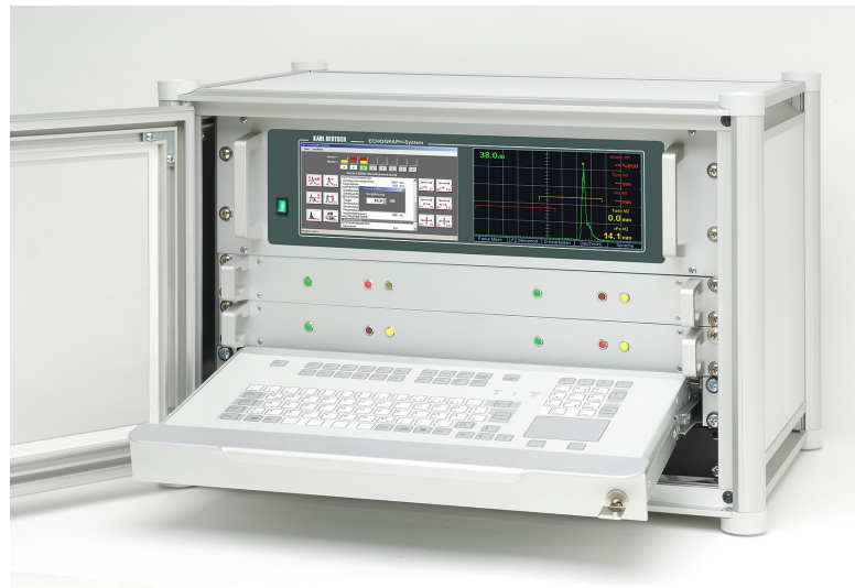
Figure Testing Electronics ECHOGRAPH 1093-testing electronics holding four testing channels which have been put into practice in the form of two double ultrasonic circuitry boards. One PC-module serves as controller for the entire system and one A-scan module represents the ultrasonic signals.
