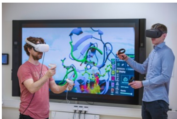
Fig. 2. Visualisation through Virtual Reality, using Oculus Quest goggles and Nanome software to explore protein structures.
