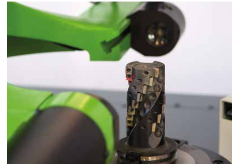
Optics carrier including CCD camera and pneumatic quick adjustment. Optional laser pointer for detection of the cutting edge.
