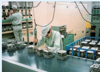
Check and repair of power meters
