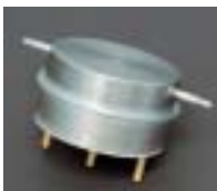
SiC diode of 6.2 kV withstand voltage
