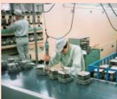
Inspect and Repair Power Meters
