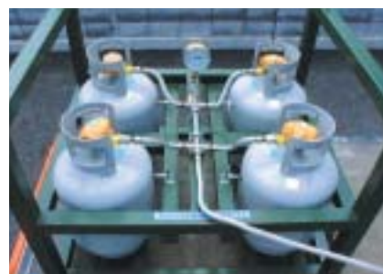
"Kankyo 1" auxiliary unit for recovering residual SF 6 gas in main system
