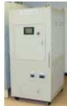
12 kVA class SiC 3-phase inverter
