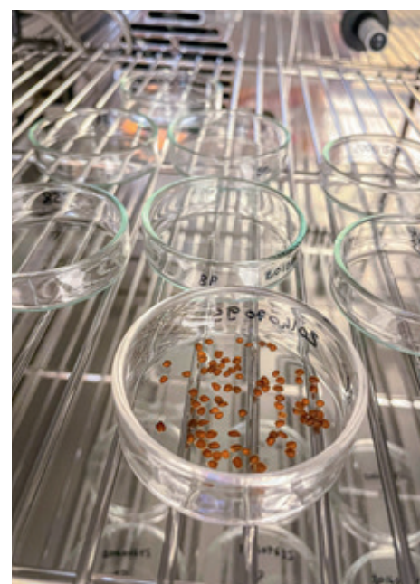
Figure 1b: Seeds in the accelerated aging treatment in a climate chamber under 40°C and 60% humidity.
