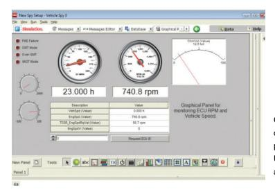
Create graphical panels to customize data display. Choose from: gauges, message panels, knobs, text boxes, buttons, and more. Users can also import custom pictures and animated components.
