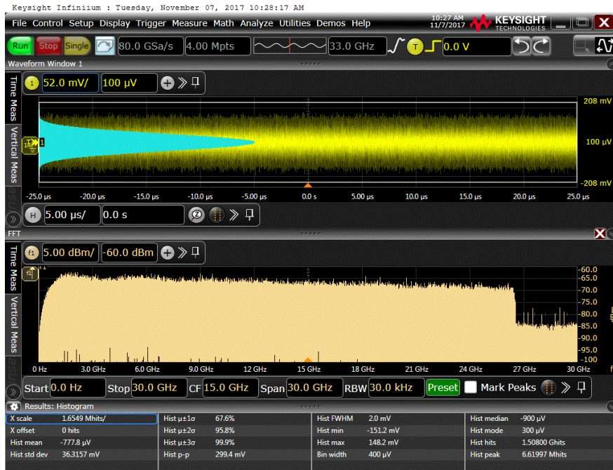
Figure 3. Random (gaussian) interference signal with a flat spectrum and bandwidth of 26 GHz, which corresponds to half of Nyquist frequency at 52 Gbaud data.
