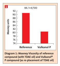
mixing problems due to high viscosity. The new processing plasticizer reduce the compound viscosity maintain other properties, as a slight polar synthetic chemical it can be expected that the material as such can improve the wet grip of a tire.
