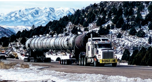
Global Specialized Services transported a demethanizer tower from Pocatello, ID to Minco, OK.
