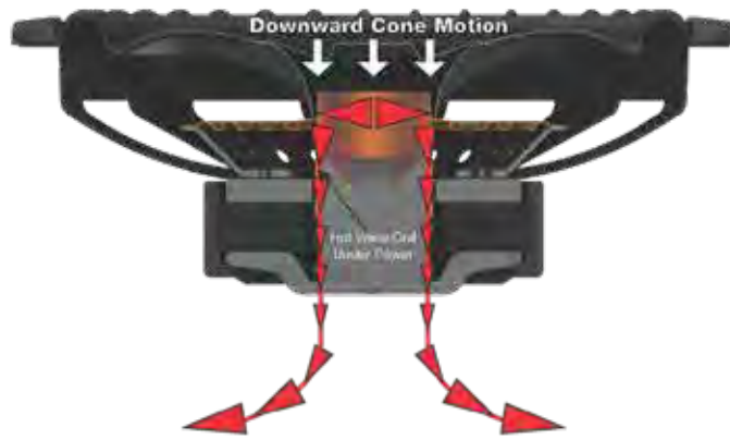
As Cone Moves Downward, Hot Air from Voice Coil is Forced out of the Woofer.
