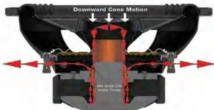
As Cone Moves Downward, Hot Air from Voice Coil is Forced out of the Woofer.
