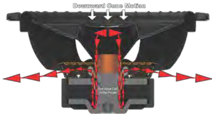
As Cone Moves Downward, Hot Air from Voice Coil is Forced out of the Woofer.
