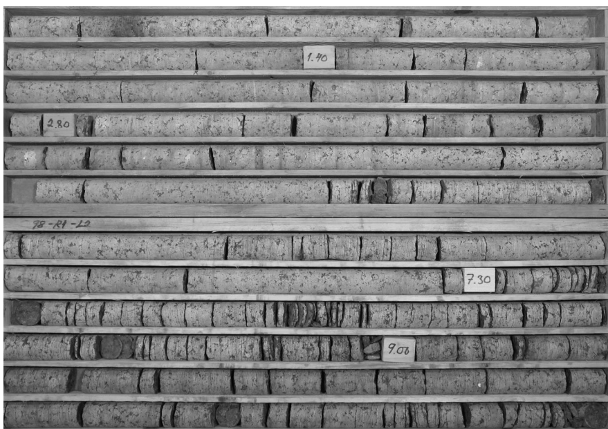
Fig. 5. Drill cores with wiborgite rapakivi granite. Wiborgite from a depth of 7.30 to 11.50 m is heavily weathered, showing intensive sub-horizontal fracturing.
