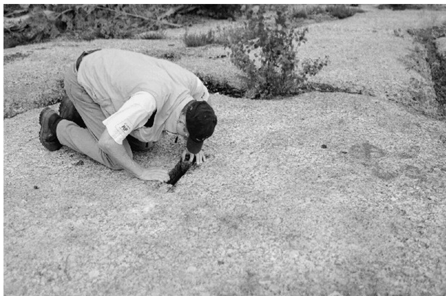
Fig. 3. Sampling was done with a hand-held diamond saw on a cleaned traverse during detailed site investigations. The sampling produced specimens approx. 7 cm in height and 20 cm in length (see Fig. 7a).
