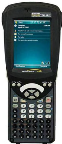
Figure 7-1: Portable (handheld) fare transaction processor used by KT and WSF for ferry fare collection
