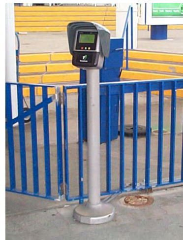
Figure 7-2: Stand alone fare transaction processor used by Vallejo Ferries in the San Francisco Bay area (similar to the ORCA ones used by Sound Transit).
