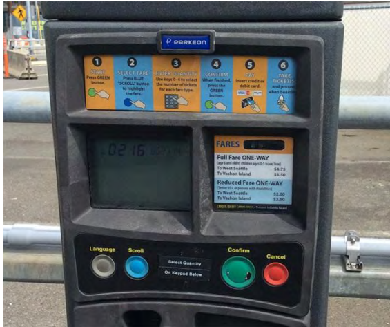
Figure 7-5: King County TVM instructions (the upper panel labeled 1 thru 6)—customers often miss these instructions and select the wrong fare
