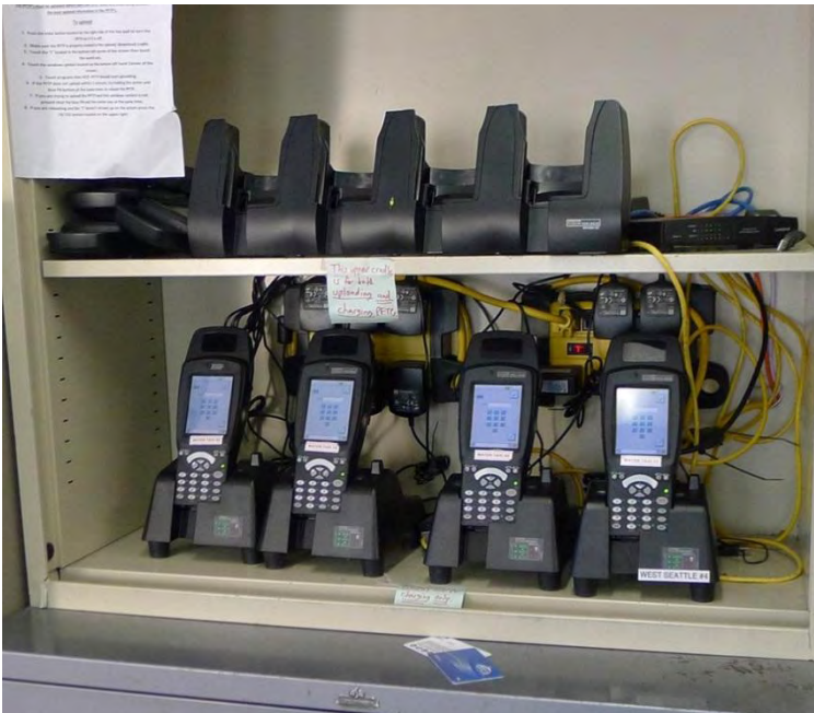
Figure 7-12: Portable fare transaction processors in charging/ communications holders (King County Water Taxi)
