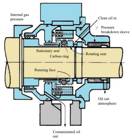
Figure 5: Mechanical (Contact) Shaft Seal
