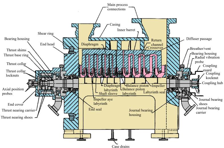
Figure 3: Centrifugal compressor nomenclature. Note: Some compressors may use bolted-head construction.
