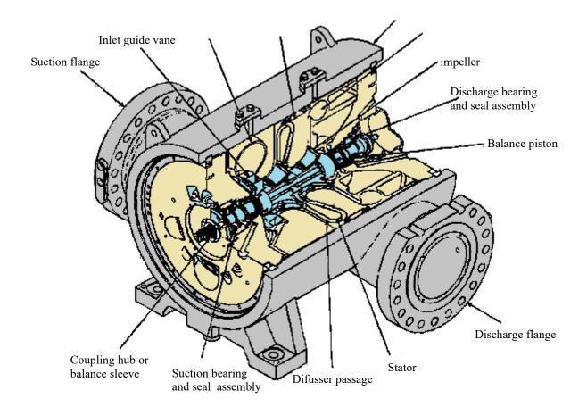
Figure 4: centrifugal compressor cut away
