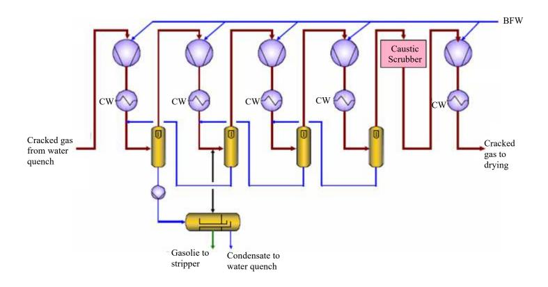
Figure 1: Conventional plant cracked gas compressor
