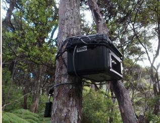
Image on left: Long-tailed bat. Image on right: Automatic bat monitor (Source: Georgia Cummings)
