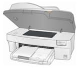
3 Wait until the printhead is idle and silent, then pinch the pinch latch on the ink cartridge with your thumb and forefinger and lift it out of the print head. Remove both ink cartridges.
