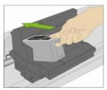
**4** Press down on the ink cartridge until you hear it snap into position.
