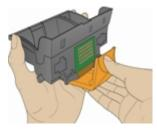
**5** Place the printhead into the carriage.
