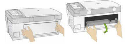
2 Insert the bottom of the duplexer into the printer and press the top in until it clicks.
