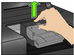
**4** Remove the old printhead from the carriage.
