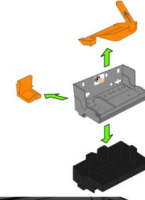
Place the new printhead into the carriage.
