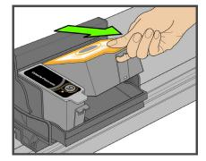
**5** Remove the bagged ink cartridge from the box, tear open the bag at the notch, and remove the ink cartridge.
