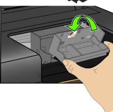
Push firmly against the target label on the printhead until it clicks into place.
