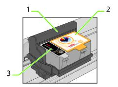
**3** Wait until the printhead stops moving, then pinch the latch on the old ink cartridge with your thumb and forefinger and lift it out of the printhead.
