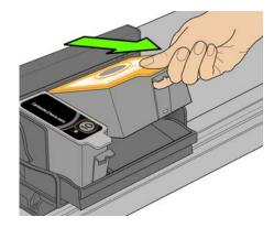
**3** Unlatch the printhead by pressing the release on the top of the carriage.
