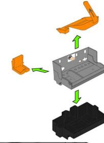
Place the new printhead into the carriage.
