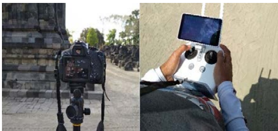
Fig.1 Using DSLR Camera (left) and Drone (right) in Acquiring Image Mosaics
