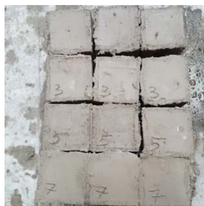
Fig. 2 The samples prepared for unconfined compressive strength tests.
