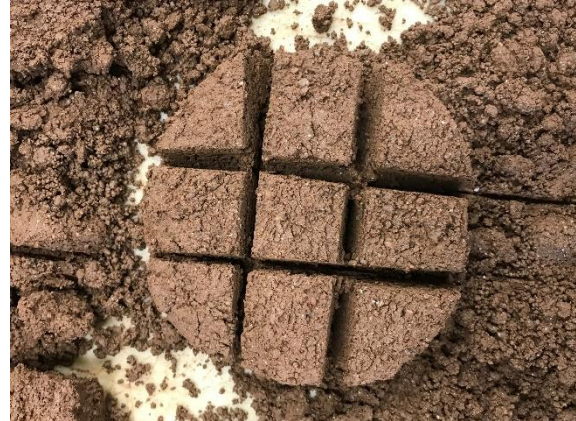
Fig. 4 Sample collection from the central part of a layer in a specimen for oven-dry weight after compaction
