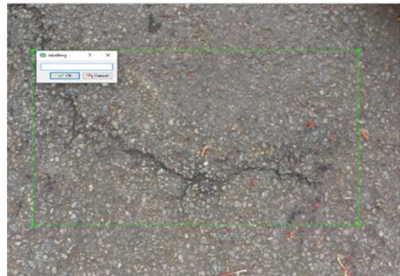
Fig.2 Example of annotation with LabelImg
