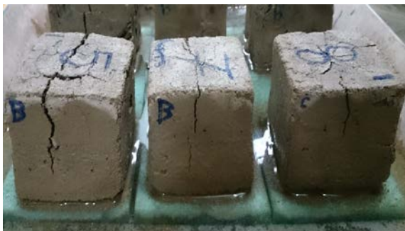
Fig. 11 The samples without reinforcement after soaked in the water for 24 hours.
