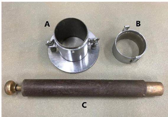
Fig.2 Standard Proctor compaction apparatus- A) Base with mold; B) Collar; and C) Rammer
