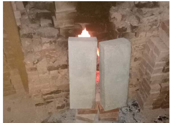
Fig. 3 The process of heating CLC bricks in a furnace.
