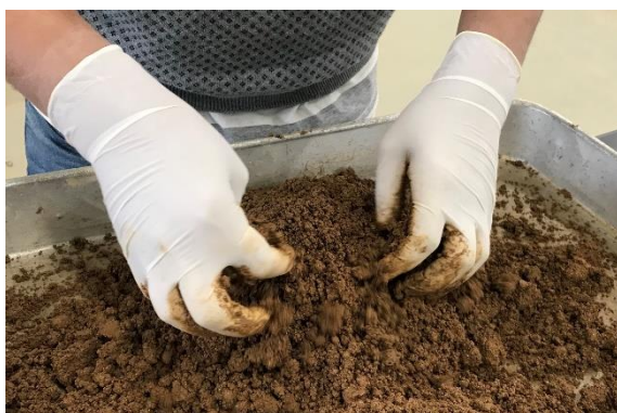
Fig. 3 Water mixing manually with air-dried soil for reaching expected water content
