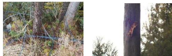
(b) Flight of PC steel stranded wire and traces of collision
