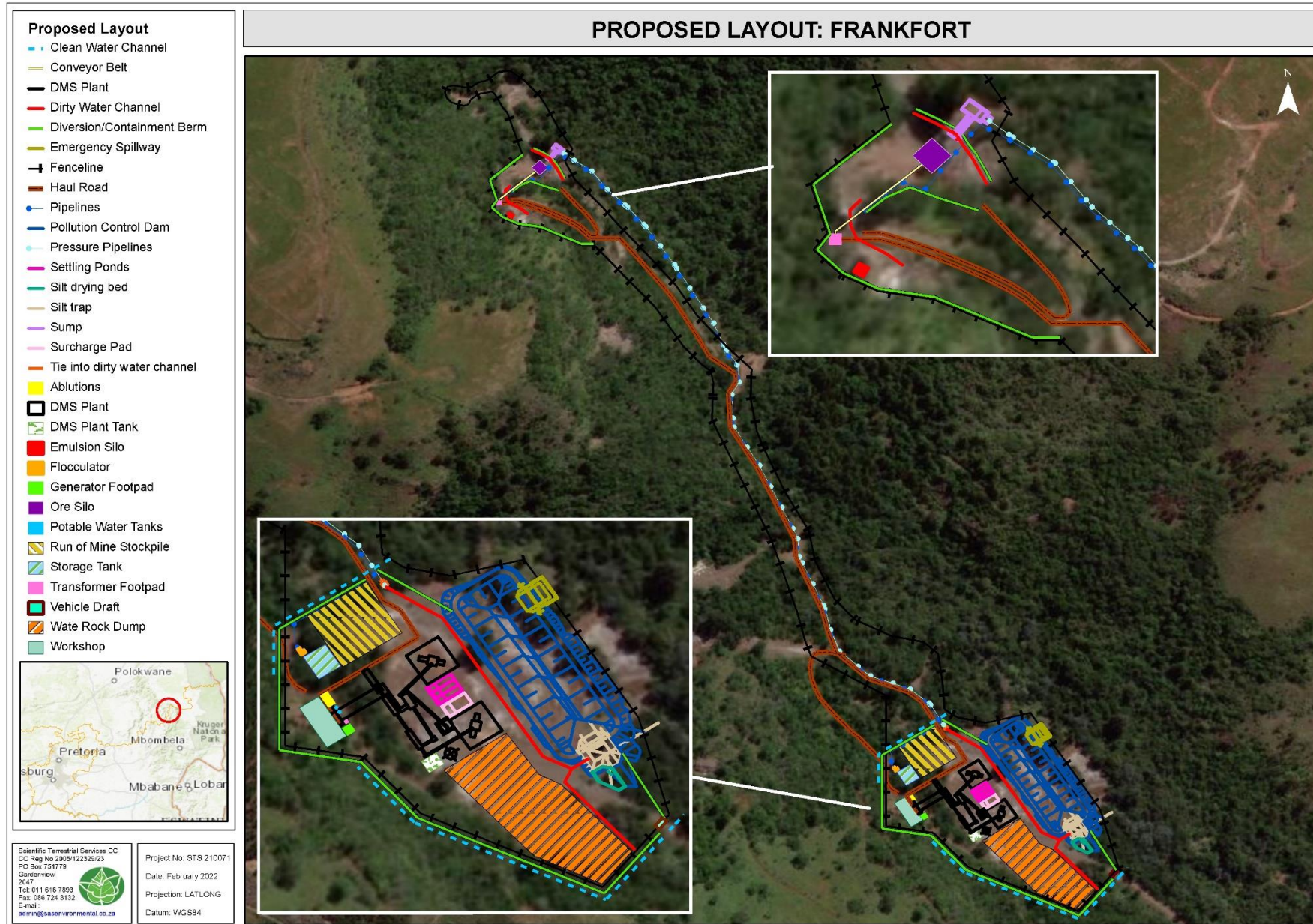
Figure 7: Proposed layout map for Frankfort provided by the EAP during the time of assessment.
