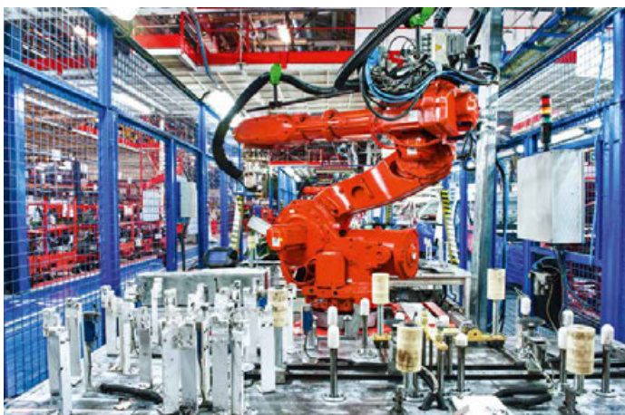
Automation for the manufacturing industry: Kontron’s IPC combined with Schleicher Electronic’s control software can operate up to 32 axes in parallel.
