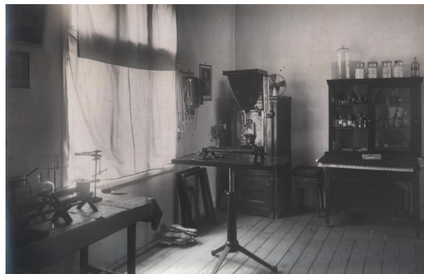
DEPARTMENT OF TECHNICAL POLICE IN BELGRADE. MICRO CAMERA, CLOSET WITH CHEMICAL PREPARATIONS, SAFE, SPECTROMETER.
