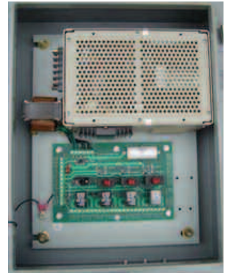
▲ Field test unit and redundant sensing and firing logic.
