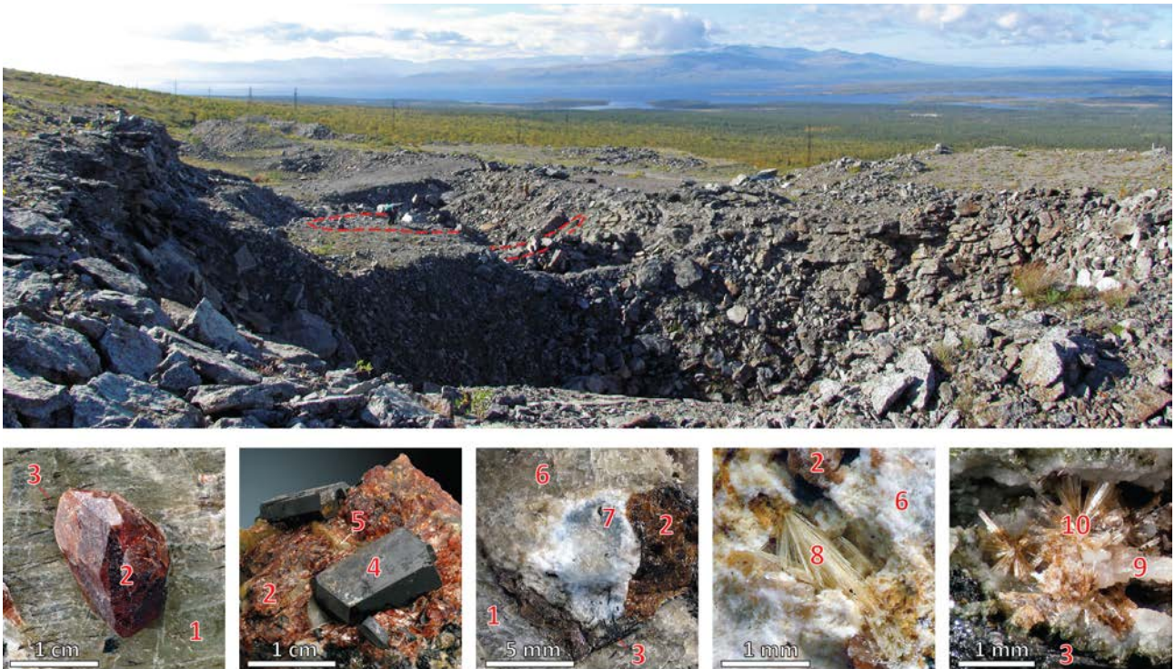
Fig. 19. The “Severny” Open Pit (Mt. Alluaiv), with the pegmatite 3-2 position. 1 – microcline; 2 – mangano-eudialyte; 3 – aegirine; 4 – magnesioarfvedsonite; 5 – nepheline; 6 – sodalite; 7 – hydroxycancrinite; 8 – eliseevite; 9 – albite; 10 – chivruaiite.
