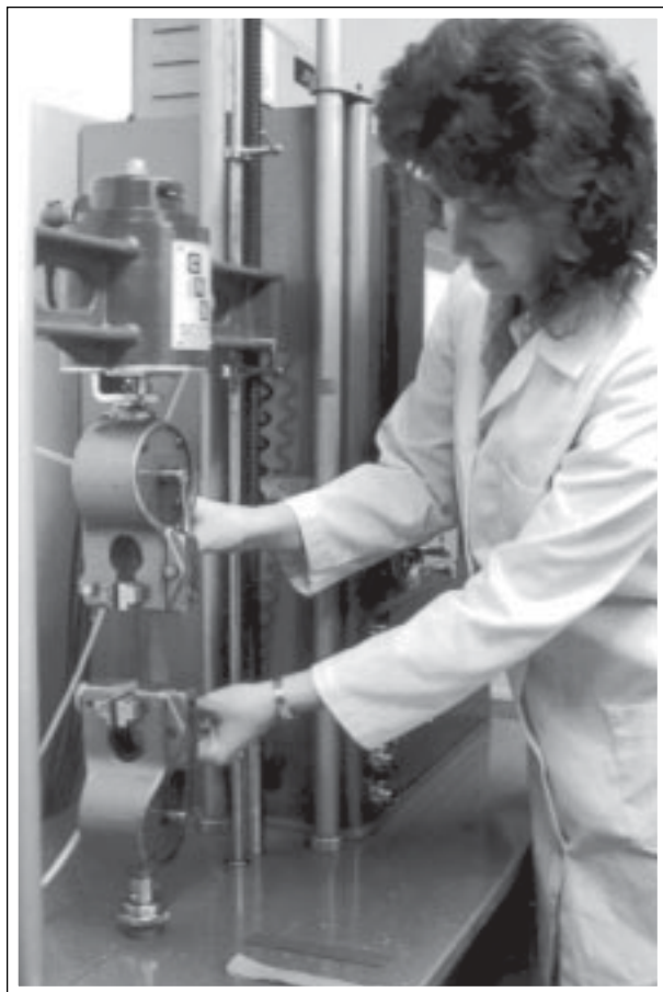
This instrument tests the breaking strength and elongation of fabrics.
