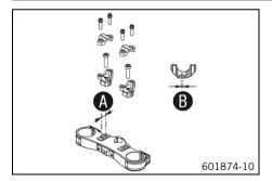
In the upper triple clamp, there are 2 drill holes separated by a distance of  $\bf A$ .
