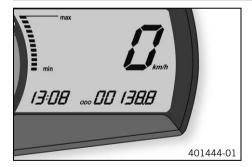
In the **0D0** display mode, the total distance traveled is shown in kilometers or miles.
