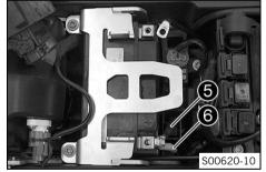
Disconnect ABS connection cable 6 and positive cable 6 from the battery.
