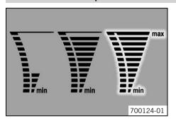
The temperature display consists of 12 bars. The more bars that light up, the hotter the coolant. When the upper bar lights up, all bars in the display begin to flash and the temperature warning lamp lights up.
