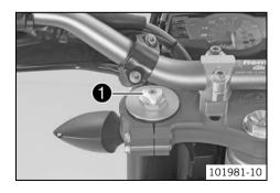
Turn the white adjusting screw 1 all the way clockwise.
