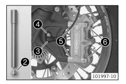
Clean and grease the thread of the wheel spindle and screw 2.
