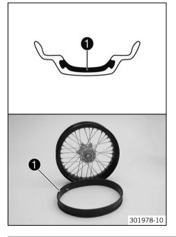
This vehicle makes use a tubeless tire system in which a tubeless sealing profile **1** is used instead of the conventional tube.
