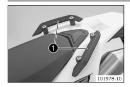
The handrails **1** are used for moving the motorcycle around. When you have a passenger, the passenger can hold on the handrails during the journey.
