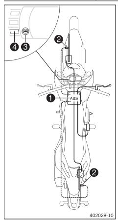
The ABS unit ①, which consists of a hydraulic unit, ABS control unit, and return pump, is installed under the seat. A wheel speed sensor ② is located at the front and rear wheels.
