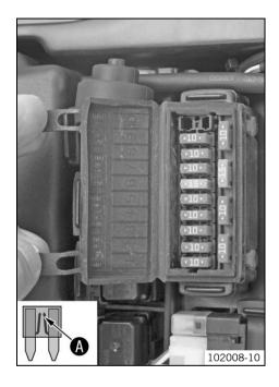
Remove the defective fuse
