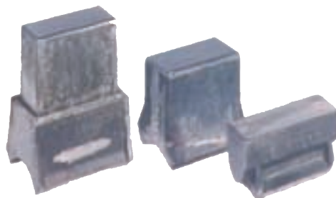
Chromium-based, high melting point skid buttons
