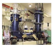
Figure 1. View of the electron cooler at S-LSR.
