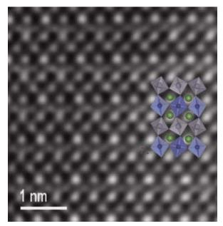
**Figure 3.** Scanning transmission electron microscope (STEM)-highangle annular dark-field (HAADF) image of the layered double perovskite LCSO film grown on the LSAT substrate.
