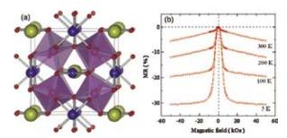
Figure 2. (a) Crystal structure of  $BiCu_3Mn_4O_{12}$ . (b) Electric resistivity in applied field at 5, 100, 200 and 300 K.
