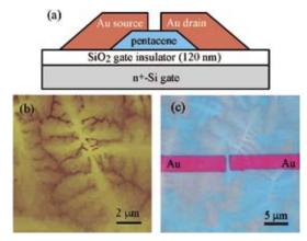
Figure 3. (a) Schematic cross section of a single-grain OFET with topcontact structure. (b) Morphology of vacuum-deposited pentacene film observed with an AFM. (c) Optical microscope image around a channel region of a single-grain OFET with 1  $\mu$ m of channel length.
