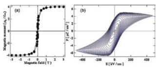
**Figure 1.** (a) Magnetization curve for  $Bi_2NiMnO_6$  film measured at 5 K which shows the ferromagnetic oredeing of  $Ni^{2+}$  and  $Mn^{4+}$  moments. (b) Ferrolelctric P-E hysterisis curve measured at 7 K.
