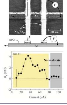
**Figure 2.** (Top) Scanning electron microscope image of a lateral spin valve device, with the geometry of the non-local measurement. (Bottom) Device cross-section.
