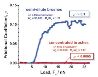
Figure 2. Plot of frictional coefficient  $\mu$  vs. load for concentrated and semi-dilute PMMA brushes in toluene.
