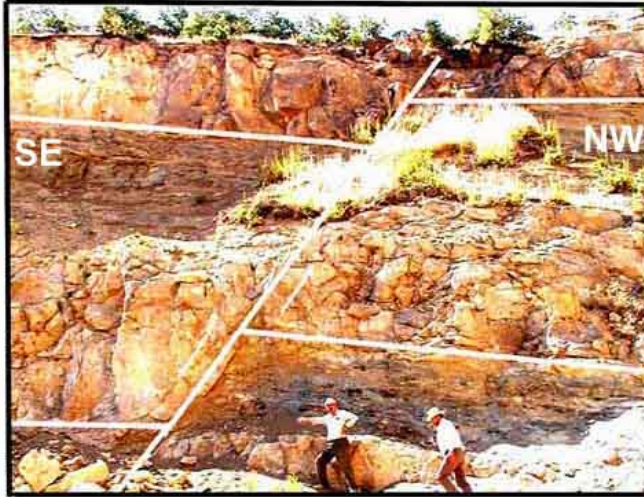
(2.1) Normal fault ( dip slip fault) at the crest of the homocline which nearly strikes parallel to slide scar.
