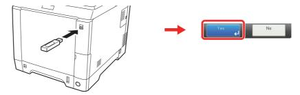
Plug the USB memory into the USB memory slot.
