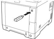
When using USB memory, plug it into the USB memory slot.
