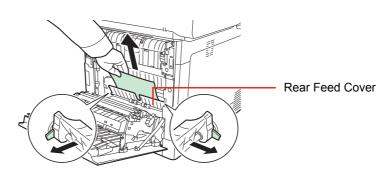
If the jammed paper is located inside the machine as shown, open the rear feed cover and pull out the paper.
