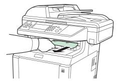
If most of the jammed paper is out in the inner tray, grasp the paper and pull it out.
