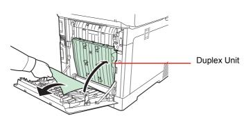
If the jammed paper reaches the Duplex Unit as shown, lift up the Duplex Unit and remove the paper.
