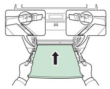
Insert the paper along the paper width guides into the tray until it stops.
