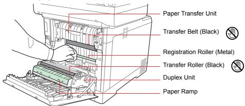
Wipe away the paper dust on the registration roller and the paper ramp using the cloth.
