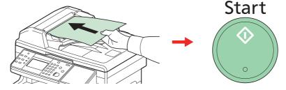
Load the original and press the Start key to start scanning.
