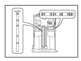
Adjust the cassette size to reflect the size of paper being loaded. Paper sizes are marked on the cassette.
