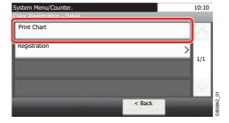
A chart is printed. On the chart, for each of M (magenta), C (cyan) and Y (yellow), charts for H-1 to 9 and V-1 to 5 are printed.
