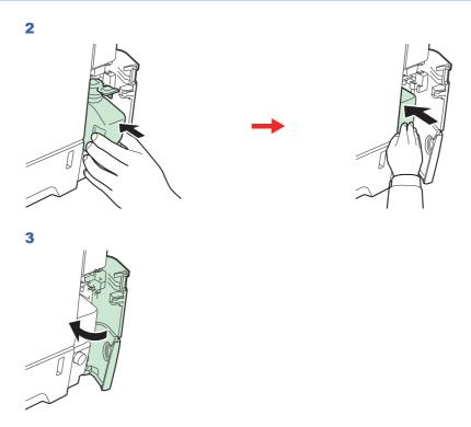
After replacing the toner containers and the waste toner box, clean the paper transfer unit. For instructions, refer to *Cleaning on page 10-6*.
