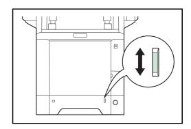
There is a paper gauge on the right side of the front of the cassette to indicate the remaining paper supply. When paper is exhausted, the pointer will go down to the level of (empty).
