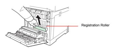
If the jammed paper does not reach the registration roller (metal) as shown, grasp the paper and pull it out.
