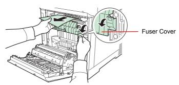
If the jammed paper reaches the fuser unit as shown, open the fuser cover, grasp the paper, and pull it out.
