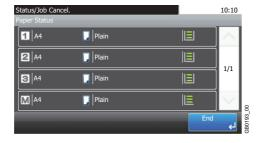
You can check the size, orientation, type, and remaining amount of paper in each paper source. The remaining amount of paper is shown by four levels as  $[]([]), []^*, []^*$ , and []([]) (none). If there is no paper in either cassette, the paper status will be shown as *No Paper*.
