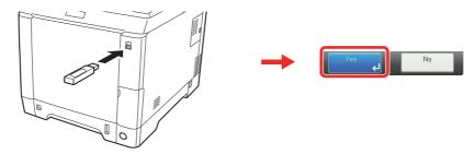
Plug the USB memory into the USB memory slot.
