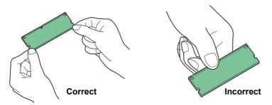
To protect electronic parts, discharge static electricity from your body by touching a water pipe (faucet) or other large metal object before handling the memory module. Or, wear an antistatic wrist strap, if possible, when you install the memory module.
