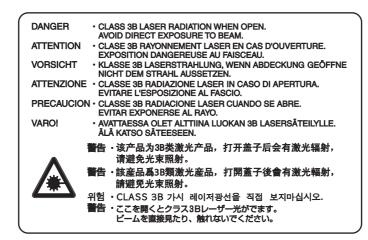
The label shown below is attached on the right side of the machine.
