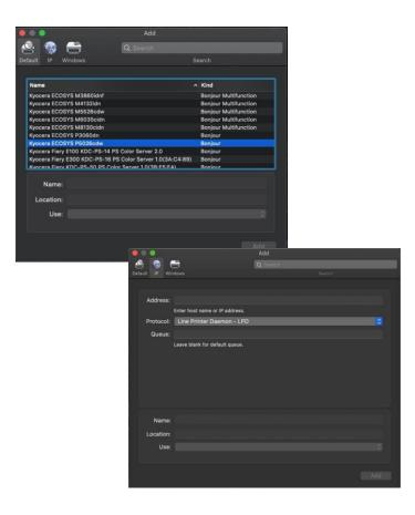
**Default**. Select the default tab. All your network and USB connected devices should appear in the window. Select your device, at this point verify in the "Use" field the correct model is selected with KPDL in parenthesis. By default, Apple selects Secure Airprint. This selection will not work correctly for our printers. Click the Use dropdown and change it to the correct PPD.
