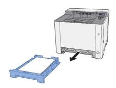
2. Remove any jammed paper. Do not reuse the jammed papers. If the paper tears during removal, be sure to remove any loose scraps of paper from inside the machine. Scraps of paper left in the device could cause subsequent jamming.
