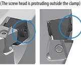
After tightening the clamp screw with the recommended torque, please check the protrusion of the clamp screw. If it is protruding outside the clamp, please reinstall
