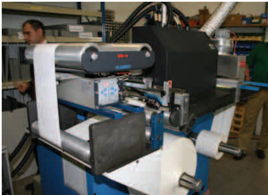
The Xaar inkjet heads mounted on the demonstration Impika UV inkjet rig
