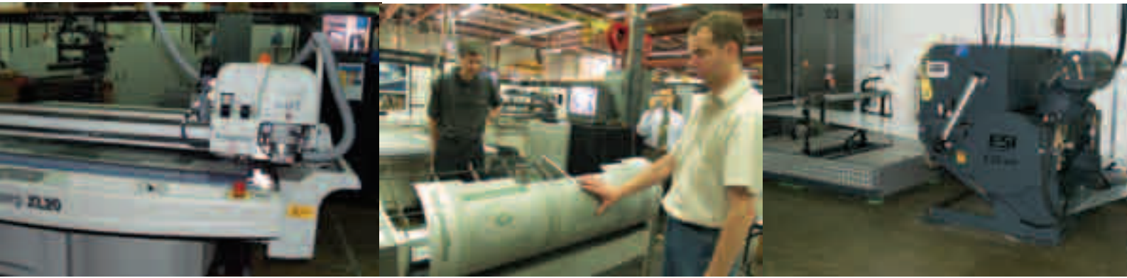
(Left-right) Plate profiles of staggered plates are cut on a Esko's Kongsberg XL20 plotter/cutter, DG's staggered plate mounting method gives a near gapless approach for continuous printing and in-line EZCure electron-beam curing unit from Energy Science Inc
