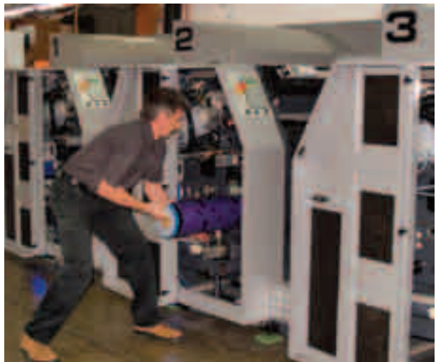
Loading an offset sleeve cylinder into one of the seven print units on the Drent Goebel VSOP
