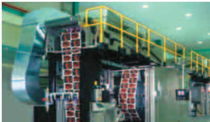
Ko-Pack STEALTH 650 16-color both sides flexo printing press
