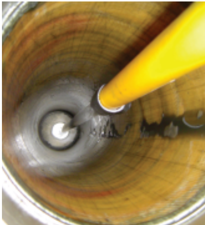
BORE cleaning w brush
