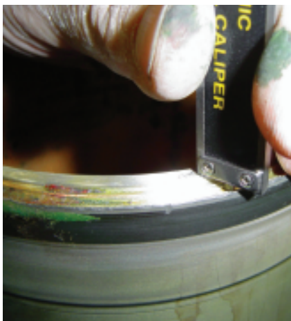
2MM worn off end of sleeve
