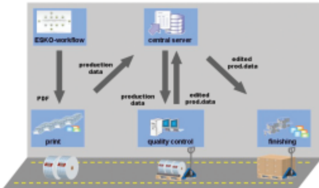
FIGURE 1 - Networking of pre-press, printing, quality control and finishing differentiated from 'acceptable' defects via a Reel Report - a
